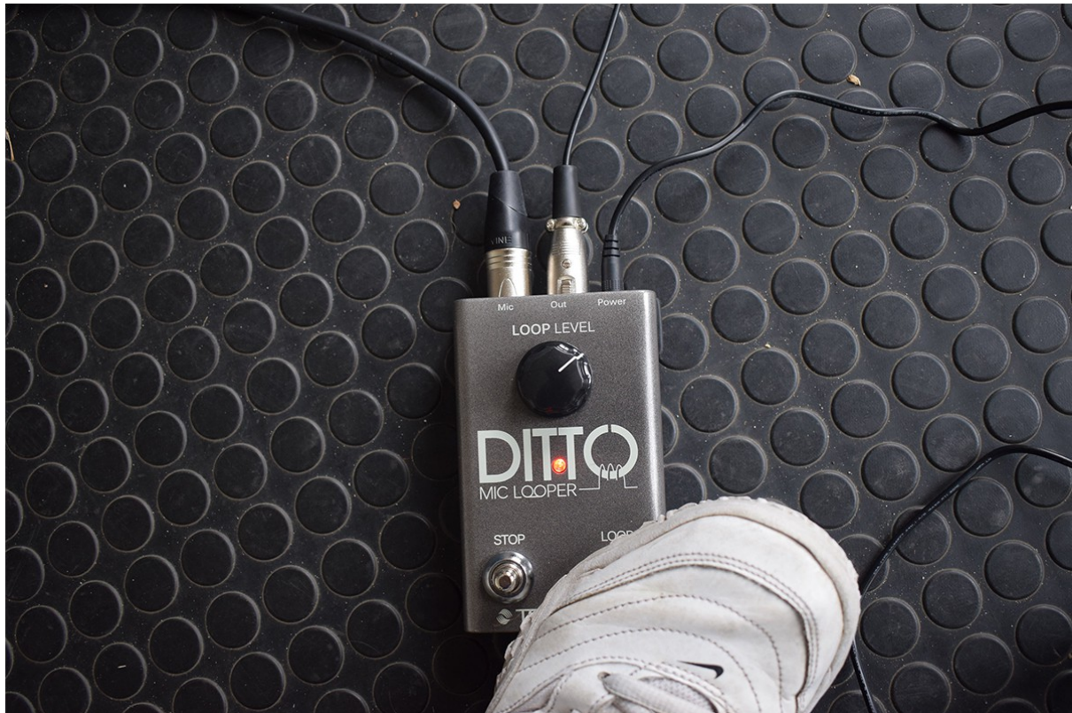
4.2 Tap the loop pedal once. The light will turn red while recording.
