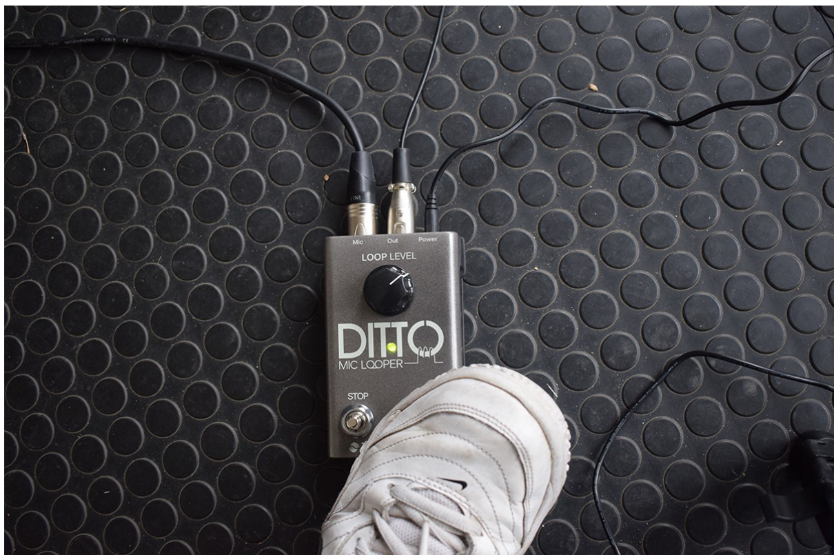
4.3 Tap again to stop the loop. The light will turn blinking green now.
